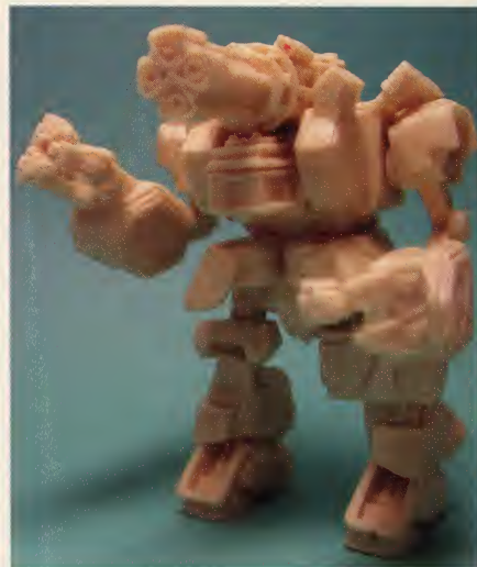
A prototype of the figure is cast using a mold made from the original sculpt.
